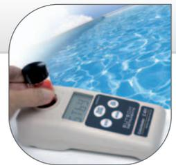
**Step 1:** To blank the meter, place a vial of sample liquid into the meter's sample well. Press the 'ZERO' button. The meter flashes 'STDBY' while blanking is in progress and displays 'ZERO' to confirm that blanking is complete
